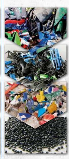
PP waste is generated as mono- or mixed fractions while sorting commercial or bulky waste. The robust and non-shreddables-resistant shredder then reliably transforms these materials into sortable flakes. Finally, they are cleaned and separated to obtain a perfect, homogeneous raw material for new, high-end products.
