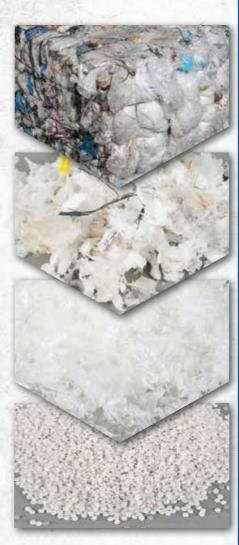
Large quantities of film find their way into the waste stream as post-consumer, post-commercial or agricultural film. They are usually contaminated with organic waste and paper labels. With modern multi-stage processing and the right washing technology, it's possible to produce clean flakes that are as transparent as possible and ideally suited to extrusion.
