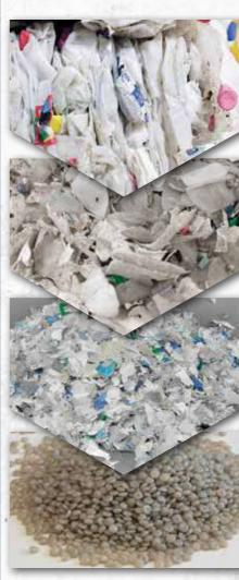
PE-HD Bottles are traded in pre-sorted and pressed form. The purity of these materials varies greatly depending on their origin. The Lindner hot-wash system produces such high-quality regrind that it can replace virgin
