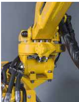
Stabilisation cylinder for sprung front axle increases stability.
