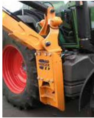
Pivot 'rotating cylinder' for narrow mounting.
