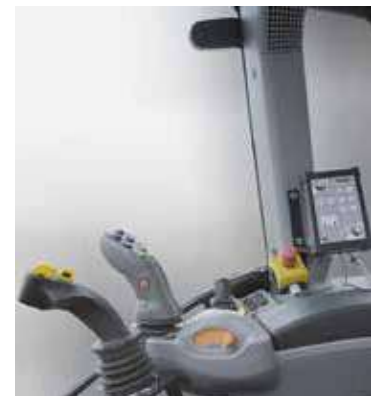
The joystick ensures accurate operation of the booms. Nivotronic is taking care of the adaption to the surface during work.
