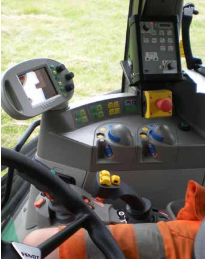
The joystick and the control box are placed in an ergonomic position.
