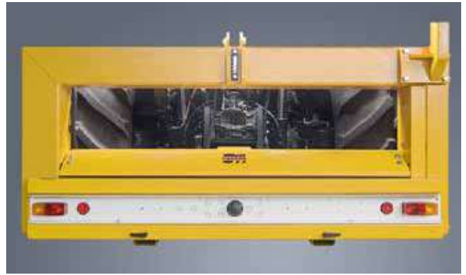
Special tank frame for the hydraulic tank keeps the top tow bar accessible for a trailer.
