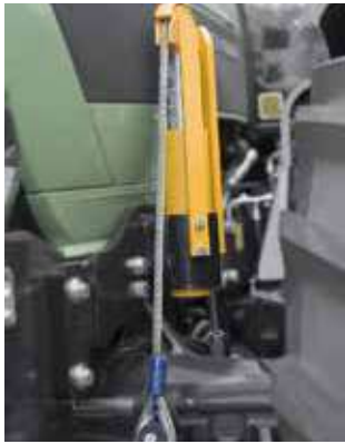
Stabilisation cylinder for sprung front axle increases stability.
