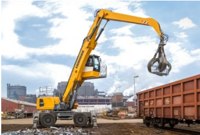
Loading extruded aluminium bundles onto wagons with the LH 50 M Industry Litronic
