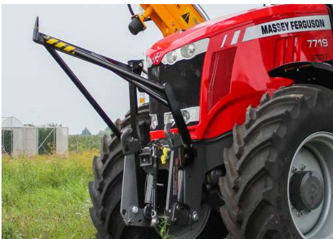
Work tool carrier on the front of the mounting frame. The boom rests on it in the transport position (MBK411).
