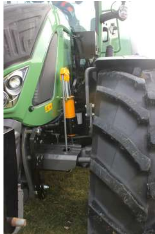
Front axle stabilisation is no luxury, but a real necessity. On the left a fixed front axle and on the right a suspended front axle.
