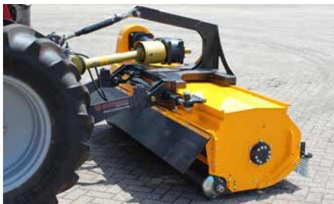
A Sideshift can be extended up to 70 cm.
