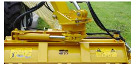
Hydraulic 180° rotating head by means of a cylinder (HD180).
