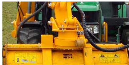
Hydraulic 180° rotating head by means of a worm gear turntable (HW180).
