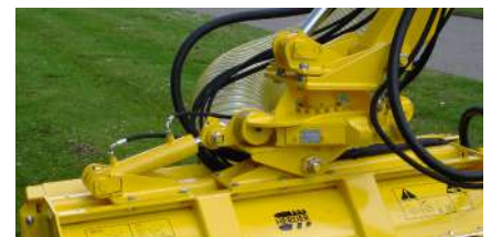
Hydraulic 180° rotating head by means of a worm gear turntable with hydraulic rod (HWHP180).
