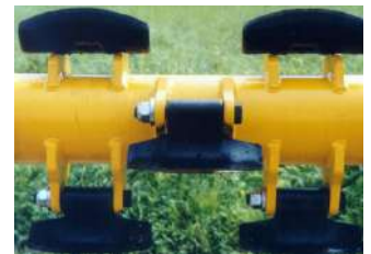
Conveyor belt unit in the heavy-duty model for grass removal when mowing ditches and slopes.
