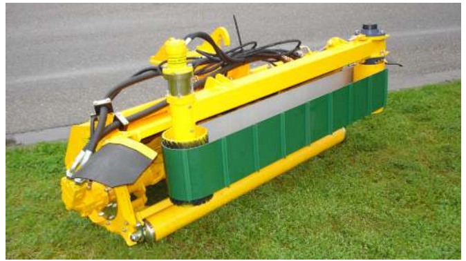
Conveyor belt unit in the heavy-duty model for grass removal when mowing ditches and slopes.
