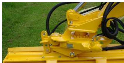
Hydraulic 180° rotating head by means of a worm gear turntable with mechanical rod (HWP180).
