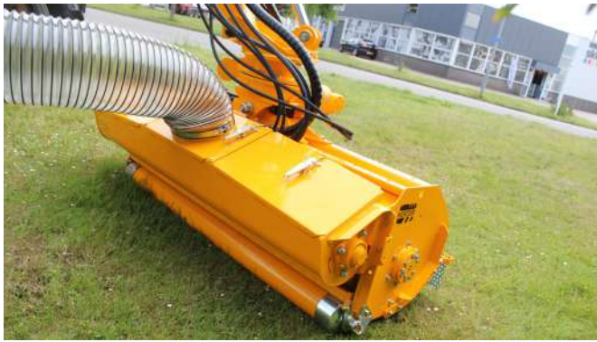
Auger unit for removing grass through suction.
