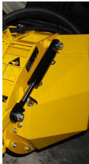
Optional motor protection and optional hydraulic folding front to feed tall plants in better.
