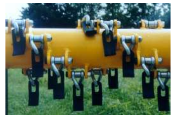
40x12 flail. This flail is suitable for mowing grass.
