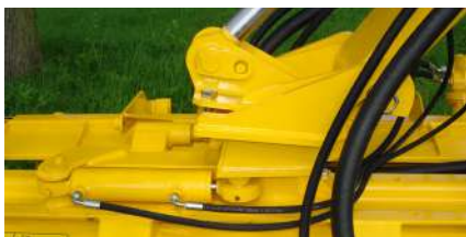
Hydraulic 90° rotating head by means of a cylinder (HD90).
