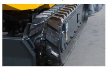
These machines are available on caterpillar tracks, or on a caterpillar undercarriage or 4-wheel model. The SCW-550H and SCW-630H models with wheels (Stump Cutter Wheeled) are supplied as standard with dual tires for extra stability and 4-wheel drive for better driving characteristics on all types of terrain. The dual tires can be removed easily, realizing a width of 85 cm for access to narrow passageways.
