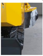
The width of the machine has been reduced to 85 cm to allow access to places that are difficult to reach. With this width, the machine can reach almost any location. Thanks to its low center of gravity, the machine is also extremely stable, despite its width.
