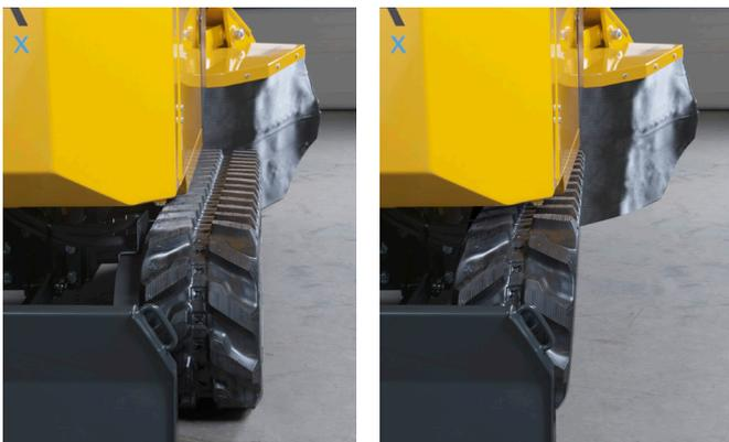
The width of the machine has been reduced to 85 cm to allow access to places that are difficult to reach. With this width, the machine can reach almost any location. Thanks to its low center of gravity, the machine is also extremely stable, despite its width.
