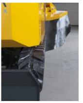
The width of the machine has been reduced to 85 cm to allow access to places that are difficult to reach. With this width, the machine can reach almost any location. Thanks to its low center of gravity, the machine is also extremely stable, despite its width.
