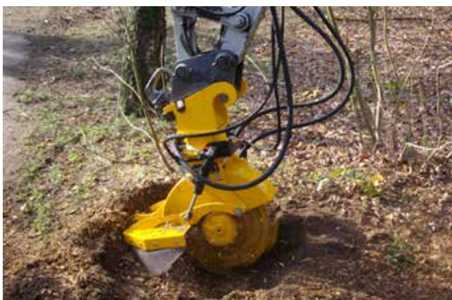
Hydraulically adjustable chip guard with SCE-410H (optional)
