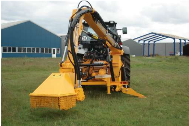
Hydraulic drive of the SC-900H
