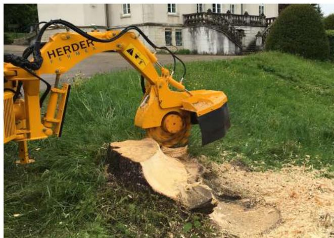
The hydraulic drive gives the cutting wheel maximum freedom of movement, as there are no mechanical constraints. The power train also has very few wearing parts so that your machine has maximum versatility.
