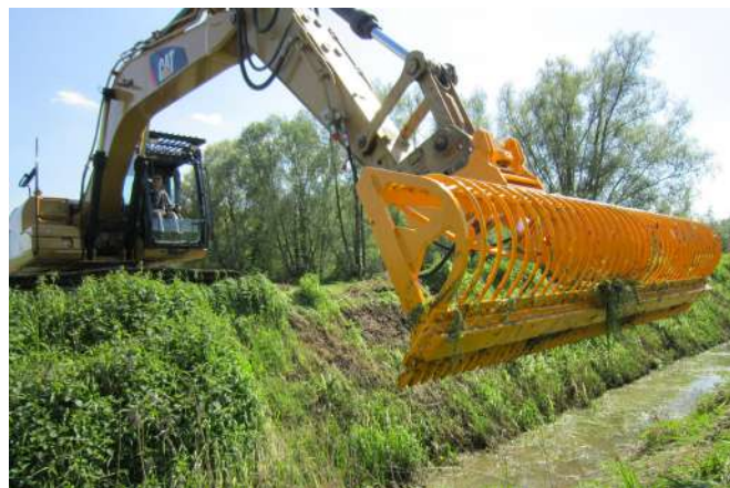
The Herder mowing bucket can be attached directly to the excavator.
